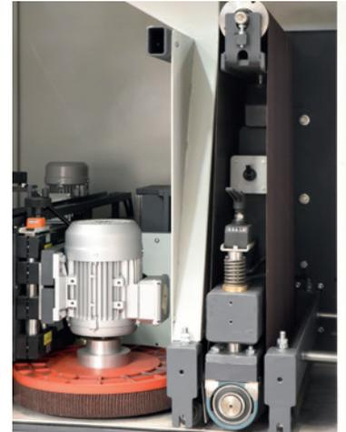
∴ With the CT650 of VG, cutted sheet parts can be deburred, edge rounded and finished in one pass. Depending on the parts to be processed (ferro-non ferro) you can choose a way to hold small parts (and if necessary large parts). This could be a magnetic or vacuum table.
